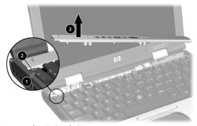
Removing the LED Switch Cover
